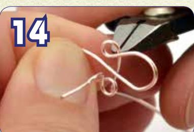
Carefully cut the loop with flush cutters. Remember to cut with the flush portion facing the wire that will remain on piece.
