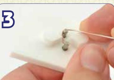
Working on the front side of the Findings Form, bend the wire to the right across the top of the peg. Wrap the wire clockwise around the peg.
