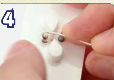
While turning the Findings Form counter-clockwise, pull and guide the wire clockwise around the peg.
