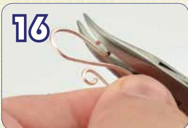
Use Bent Chain Nose Pliers to completely flatten the small loops. Make sure they are flat and closed.
