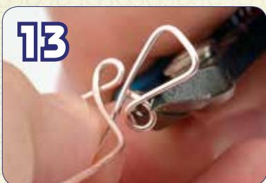
Trim one loop by facing the flush side of the Flush Cutter toward the wire that will remain on the piece, and cut the remaining excess wire.
