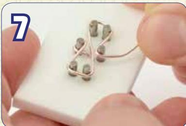
Pull the wire in between the center two pegs, and wrap counter-clockwise around the right peg.
