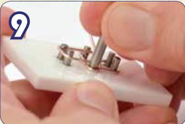
Use the pusher tool to mash each of the intersections of the wire. This helps to flatten the entire piece.
