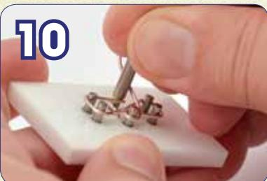
Push the wire all the way down with the Pusher tool.
