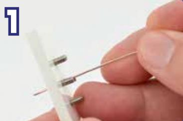
Cut a 4 1/2" (11.4cm) length of 18, 20 or 22 gauge Artistic Wire, and insert one end into the hole in the center of the Findings Form about 1/4" (6mm).
