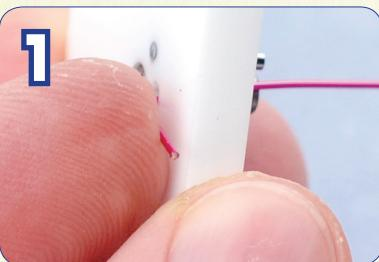
Insert a piece of wire (20-24Ga) 5" (12.7 cm) in length through the hole in the Findings form and bend the end (this helps to hold the wire firmly as you bend the wire around the pegs).
