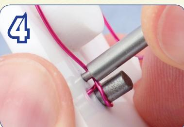
Use the Pusher tool on the small peg to tighten the intersection of the wire.
