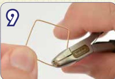
Use the Bent Chain Nose Pliers to flatten the loop.
