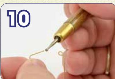
Insert the tip of the ear wire onto the end of the Wire Rounder. Spin the Wire Rounder until the sharp edge is completely smooth.
