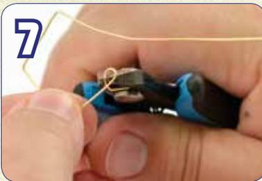
Trim the loop by facing the flush side of the Flush Cutter toward the ear wire and cut the remaining excess wire.
