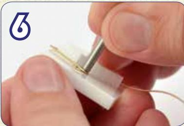
Use the pusher tool over the metal peg to mash the loop. Unbend the beginning end of the wire from the back of the Findings Form and push the ear wire off.
